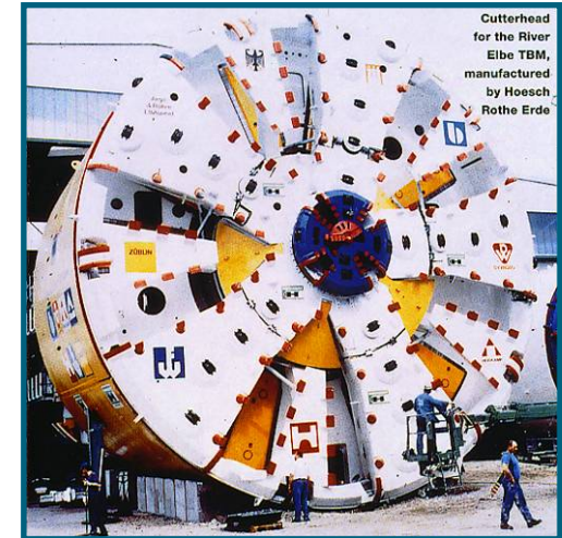
Elbe Tunnel Slurry Machine
