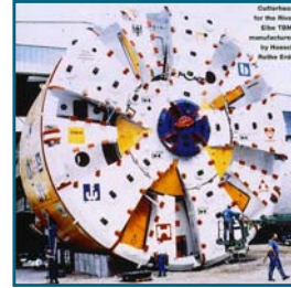
Elbe Tunnel Slurry Machine
