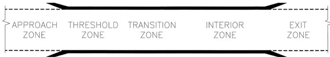
Figure 3-5. Tunnel Lighting Zones
