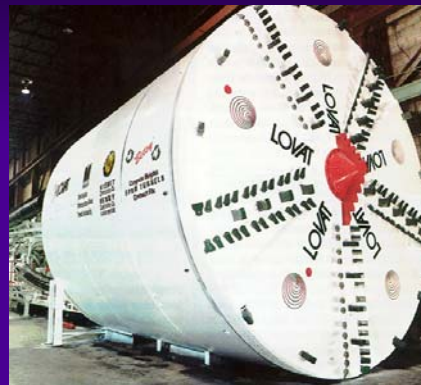
6.45m Open/EPB TBM - Contract F6c
