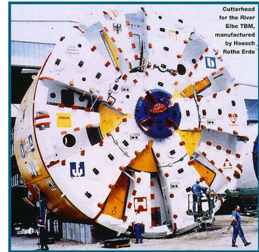
Elbe Tunnel Slurry Machine
