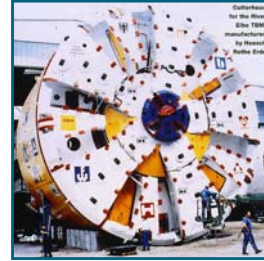
Elbe Tunnel Slurry Machine
