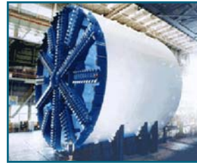
Seven tunnel boring machines will be used in the Madrid Calle 30 project
