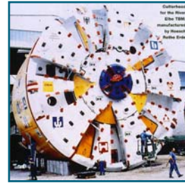
Elbe Tunnel Slurry Machine
