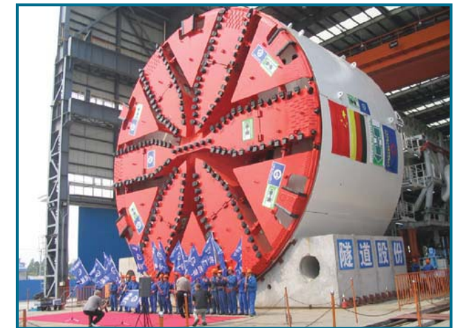
This tunnel boring machine is 50.6 feet in diameter and is similar in size and type to the machine we will use to create the SR 99 bored tunnel.
