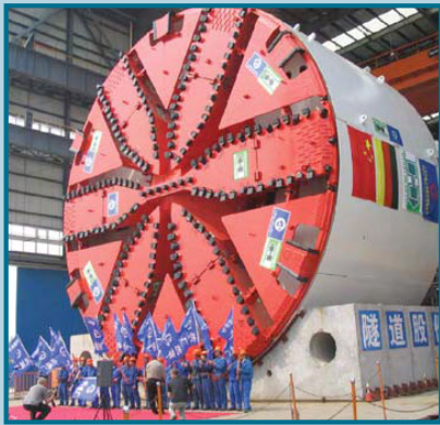
This tunnel boring machine is 50.6 feet in diameter and is similar to the machine we will use to create the SR 99 bored tunnel.
