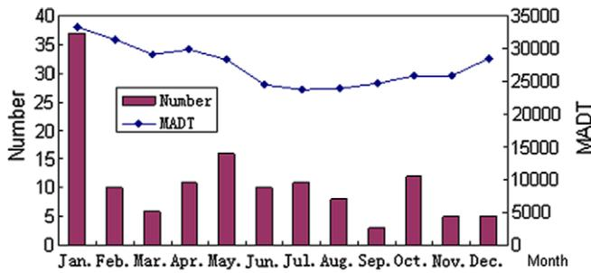
Fig. 3. Monthly distribution of traffic accidents in tunnels.
