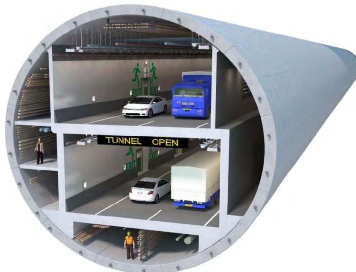
Figure 12: Conceptual Bored Tunnel Cross-Section
