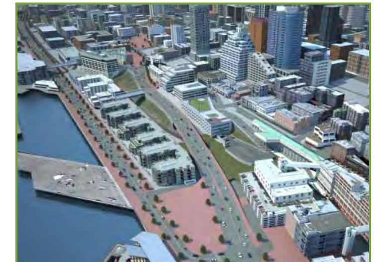
The north end of the waterfront roadway would connect over the railroad tracks to Elliott and Western avenues. This is a view of the roadway looking north toward Belltown.
