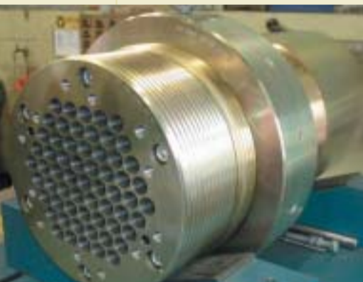
A stay cable anchorage point.
